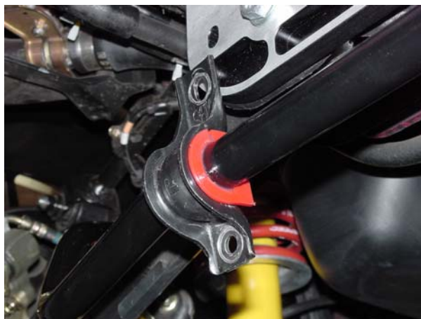
8. Position bar on end links and install nuts. Torque to 38Nm (28 lbf ft.) Apply supplied grease to inside of bushing and install bushing and mounting clamp onto bar. (Left side shown, repeat for right side)
