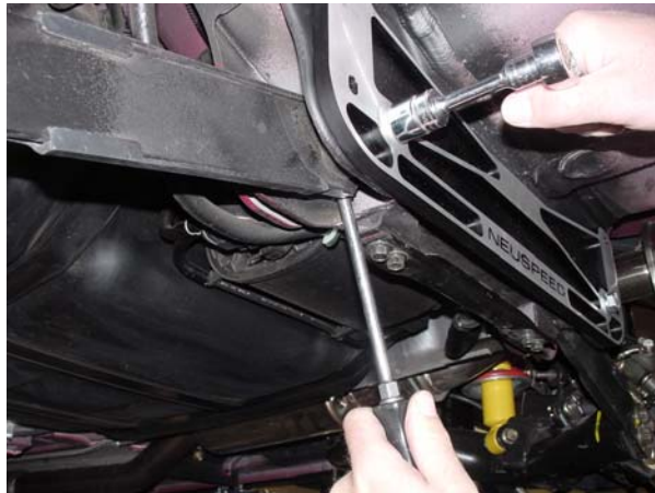
7. With a pry-bar, position lower control arm and thread bolt (19mm hex) into sub-frame. Do not tighten completely. (Left side shown, repeat for right side)
