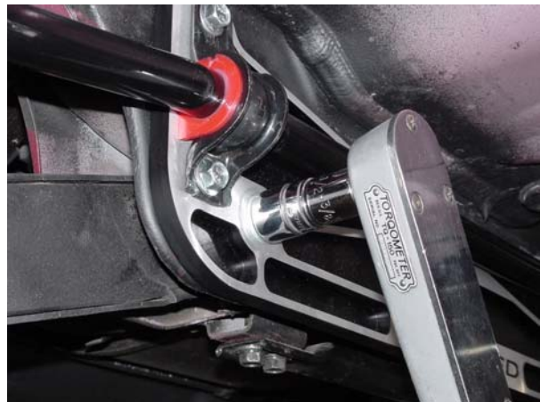
10. Lower vehicle onto ground and torque control arm bolts to 59Nm (43 lbf ft.) (Left side shown, repeat for right side)
