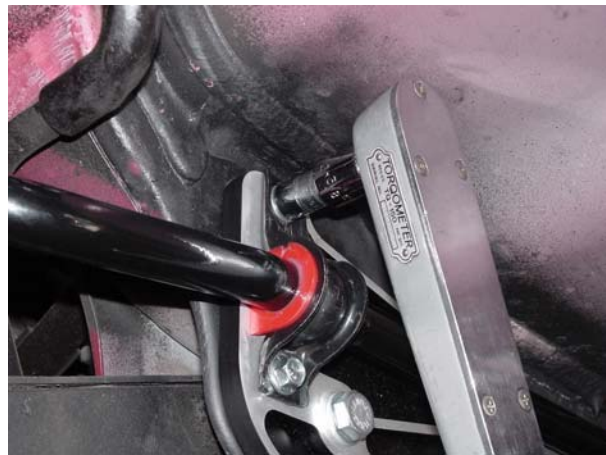
9. Rotate bar up to mounting plate and install mounting bolts (12mm Hex) as shown. Torque bolts to 22 Nm (16 lbf ft.) (Left side shown, repeat for right side)
