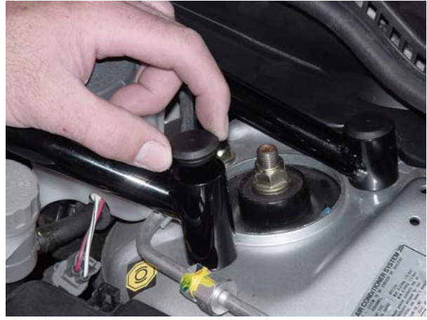
6. Install caps on strut bar ends.
