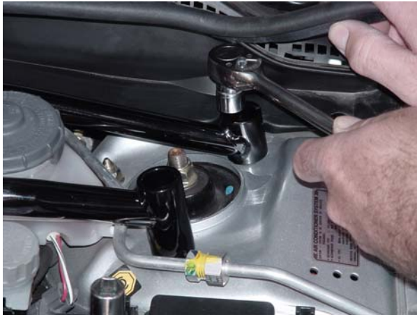
4. Start each retaining nut by hand, then torque to 33 ft. lbs. Note: Install rear driver side nut by hand with 14mm deep socket then torque to 33 ft.lbs. with standard socket.
