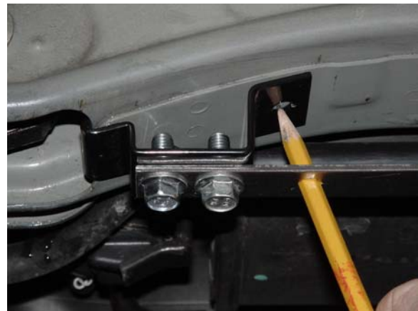
4. Using the installed bracket as a template, mark the sub-frame with a pencil. (Left side shown. Repeat for right side)
