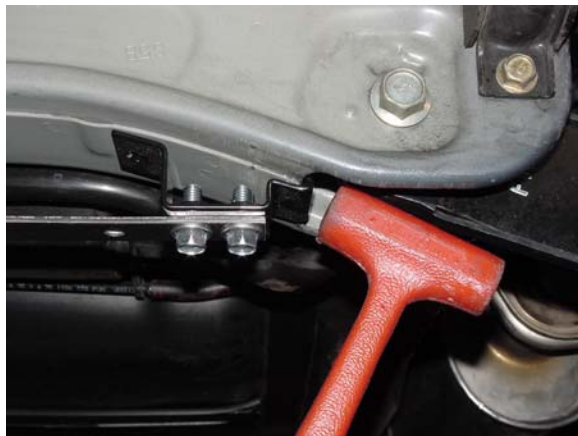
2. Seat bracket against seam of bulkhead by striking with dead blow hammer in area shown. (Right side shown)
