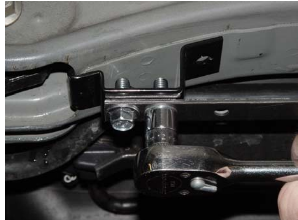
3. Insert left side bracket and repeat step #2. Install M8 bolts using 12mm socket as shown.
