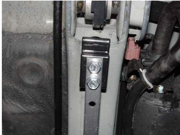
1. Position assembled bracket as shown and slide onto bulkhead seam. (Right side shown)
