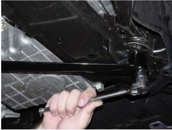
6. Torque all bolts to 76 ft./lbs. (98Nm).
